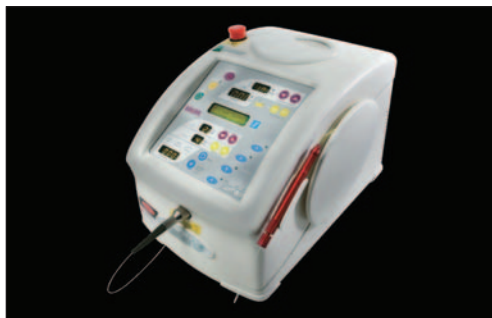
Fig. 22 Example of a 'desktop' diode laser machine. Common wavelengths are KTP (532 nm), diode (810 nm) and diode (980 nm)
