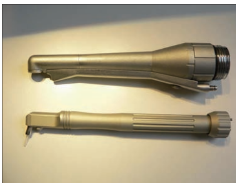
Fig. 14 Top: early Er:YAG hand-piece; bottom: current hand-piece, which is lighter and more accurate in use
