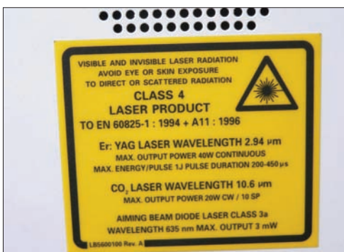
Fig. 9 Back-plate, Er:YAG/CO 2 laser
