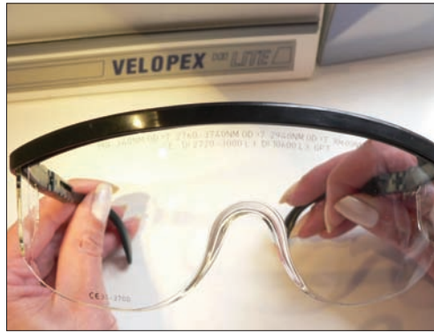
Fig. 16 CE mark and OD values for wavelength protection (>5.0)
