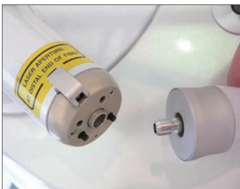
Fig. 11 Designated delivery system with unique interlock/wavelength
