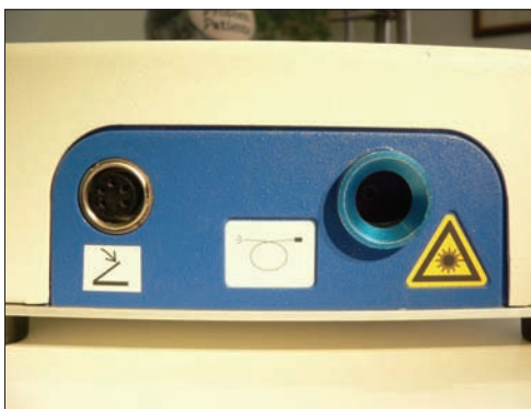
Fig. 7 Ports for foot-pedal and fibre
