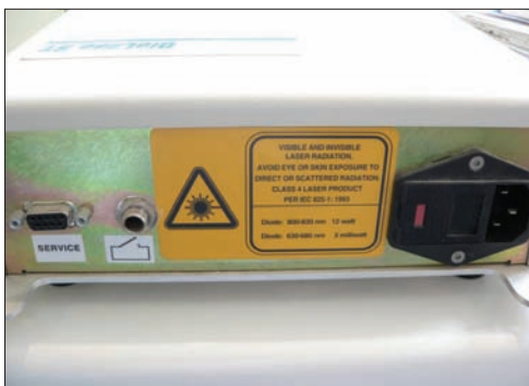
Fig. 8 Backplate, diode 810 nm laser, showing service port, remote interlock port and mains electricity socket (fused)
